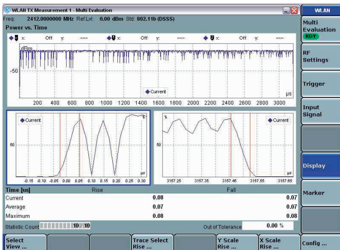
FIG 1 The power vs. time measurement graphically displays the measured transmit power over the duration of a burst. The transmit power-up and power-down ramps are of particular interest. For DSSS signals in line with IEEE 802.11b, section 18.4.7.6 specifies the time for the burst to transit from 10 % to 90 % or 90 % to 10 % of linear power.
