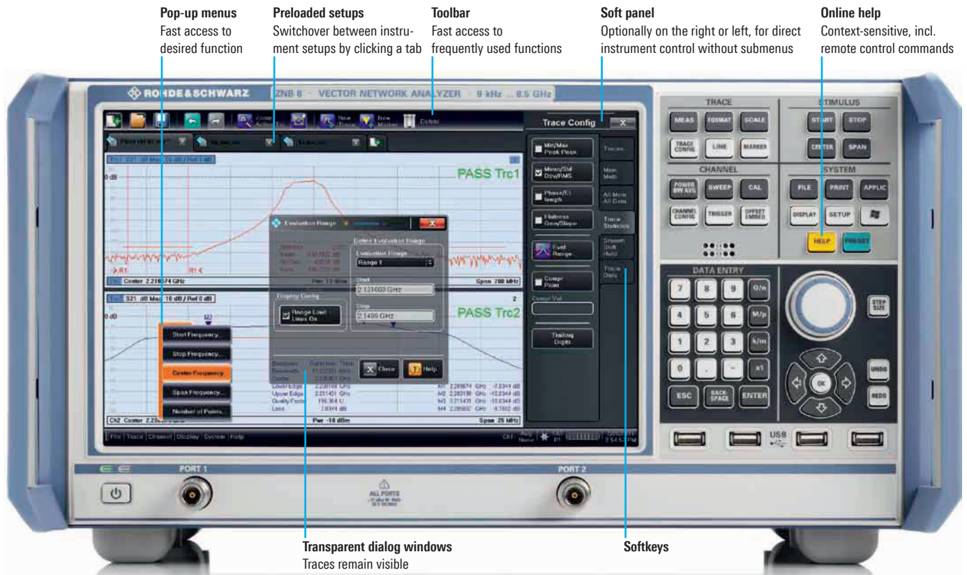
FIG 2 The R&S®ZNB and R&S®ZNC provide truly intuitive measurement and analysis. Basic functions are operated via hardkeys; all other functions are controlled via the 30 cm (12.1") touchscreen. Submenus and multilevel, nested menu structures are not needed.
