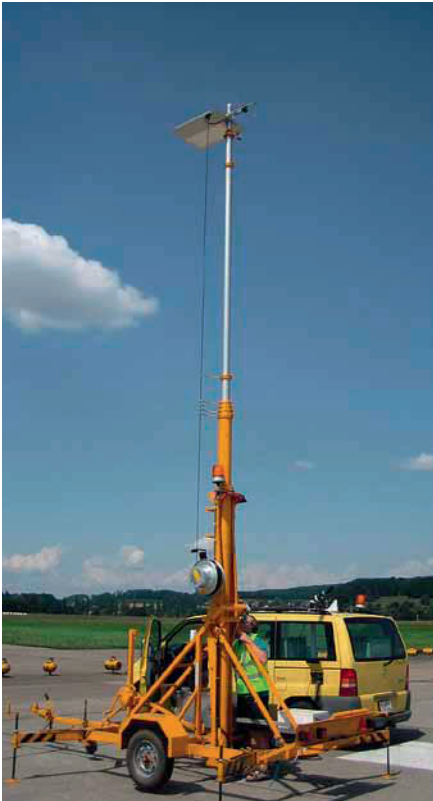
FIG 7 Telescopic mast for glide path measurements.
