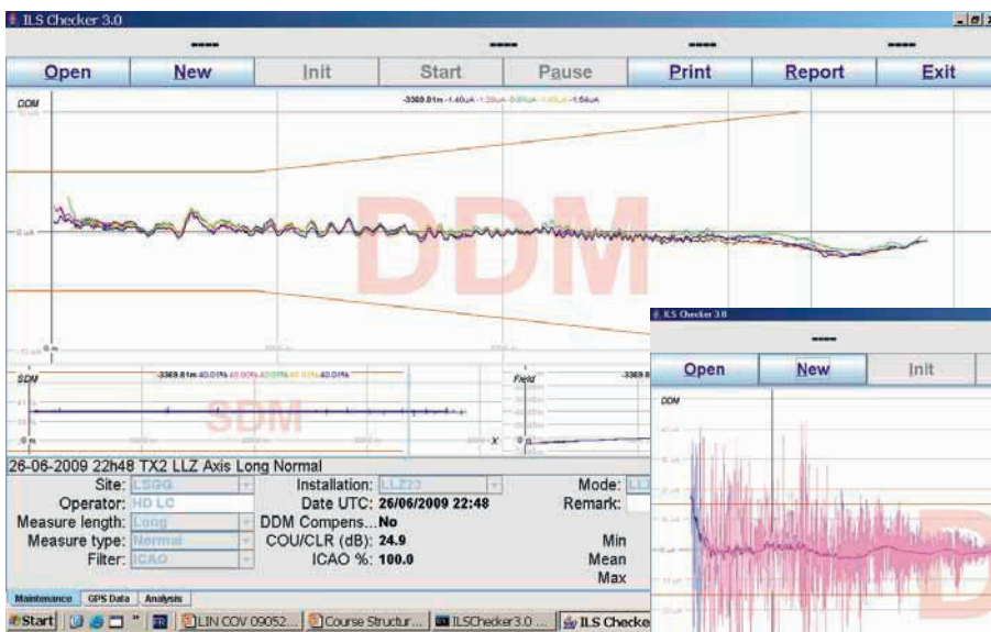
FIG 3 Course structure measurement with reference traces.
