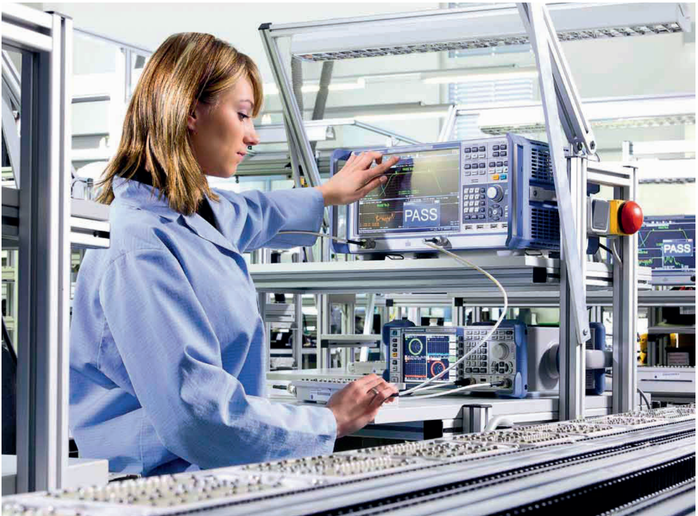
FIG 1 The R&S®ZNB8 (top) and the R&S®ZVL vector network analyzers (bottom) in a production environment.
