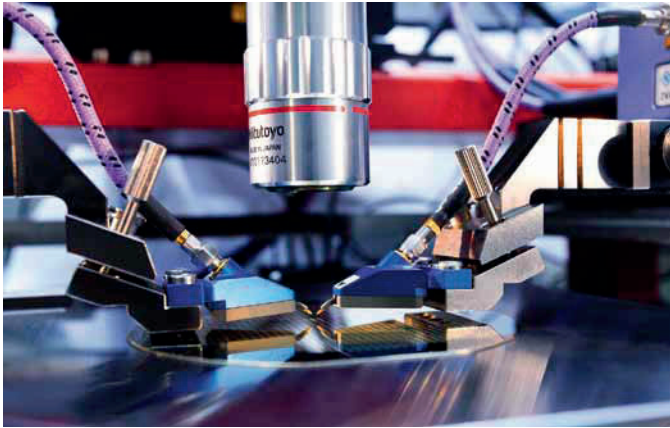
FIG 3 Test setup with diplexers, 1 mm coaxial cables and probe tip.
