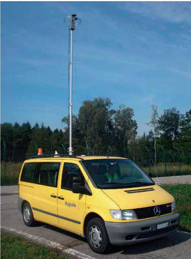
FIG 1 Vehicle with built-in telescopic mast for localizer measurements.
