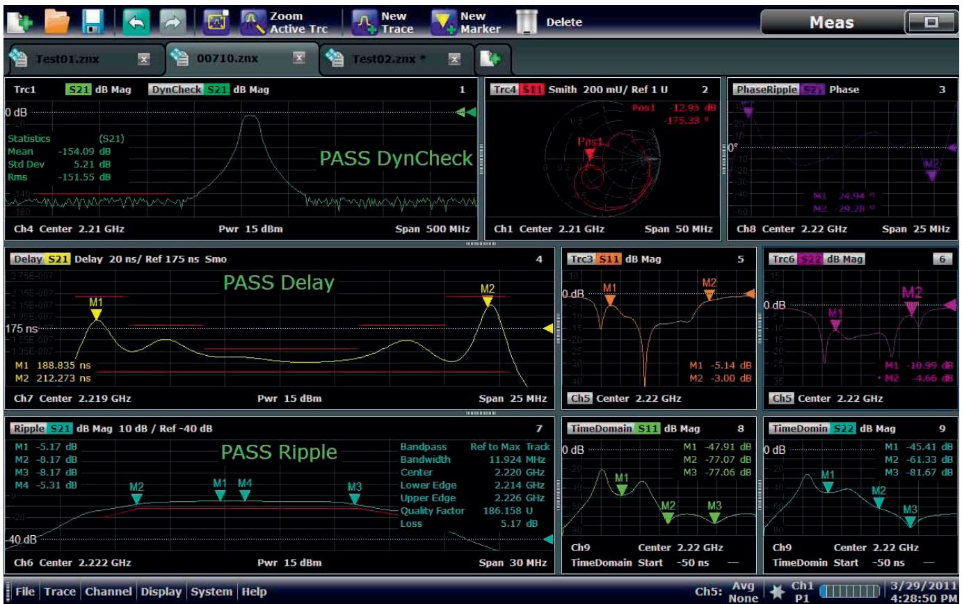
FIG 3 The soft panel can be hidden, leaving the full screen area for the display of results.
