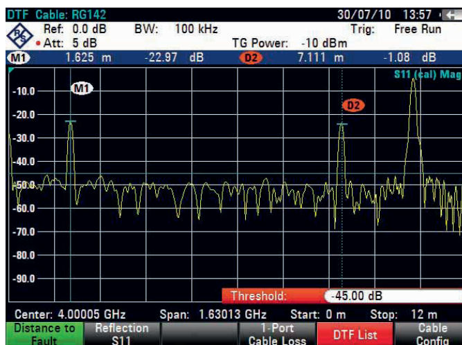
FIG 5 Distance-to-fault (DTF) measurements can be used to quickly locate damage.
